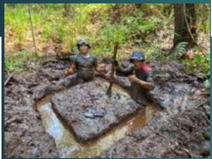
Trenched plot – isolates emissions from peat
